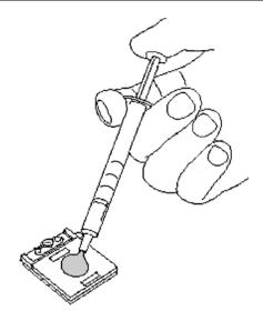
Figure 4-30 Applying new grease
